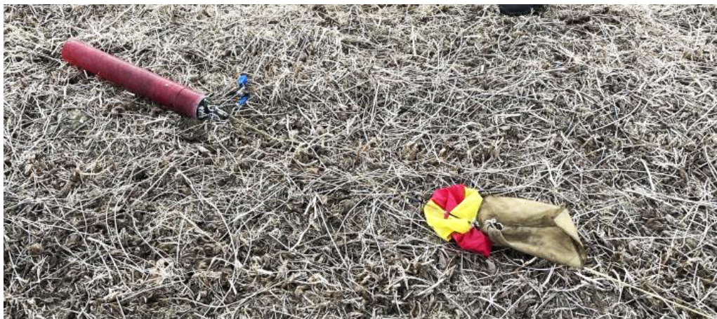
Figure 3.28: Subscale avionics section with attached shock cable and drogue parachute as landed
