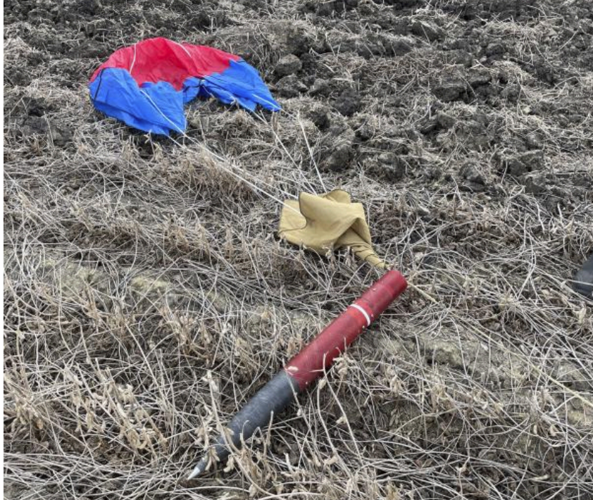
Figure 3.29: Payload and nose cone section with attached shock cord and main parachute as landed. Bearing seen here as a white stripe
