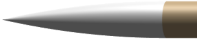
Figure 3.5: Example of a long-ogive nose cone
