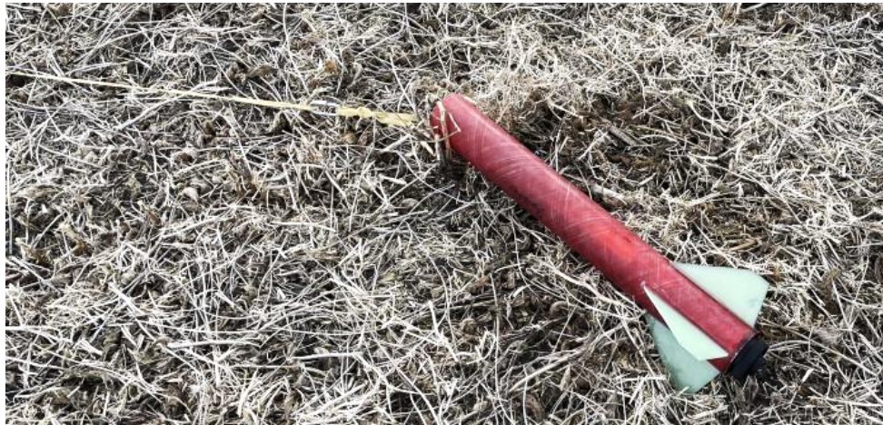
Figure 3.27: Subscale booster section with attached harness as landed
