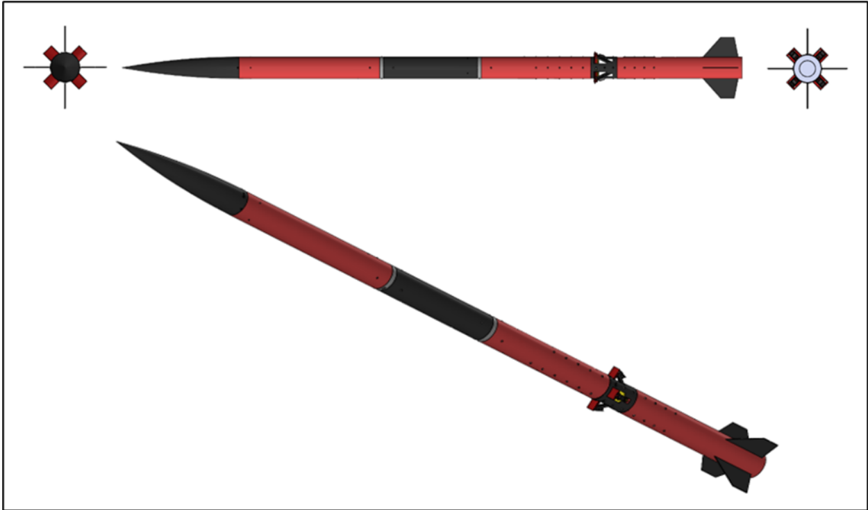
Figure 3.1 Full-Scale CAD Model: Three View
