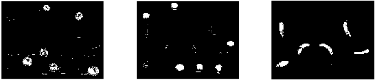
Figure 7: Image of masks2.png with correctly classified fruits and noise. Shown from left to right: apples, oranges, bananas from mixed_fruit2.tiff.
