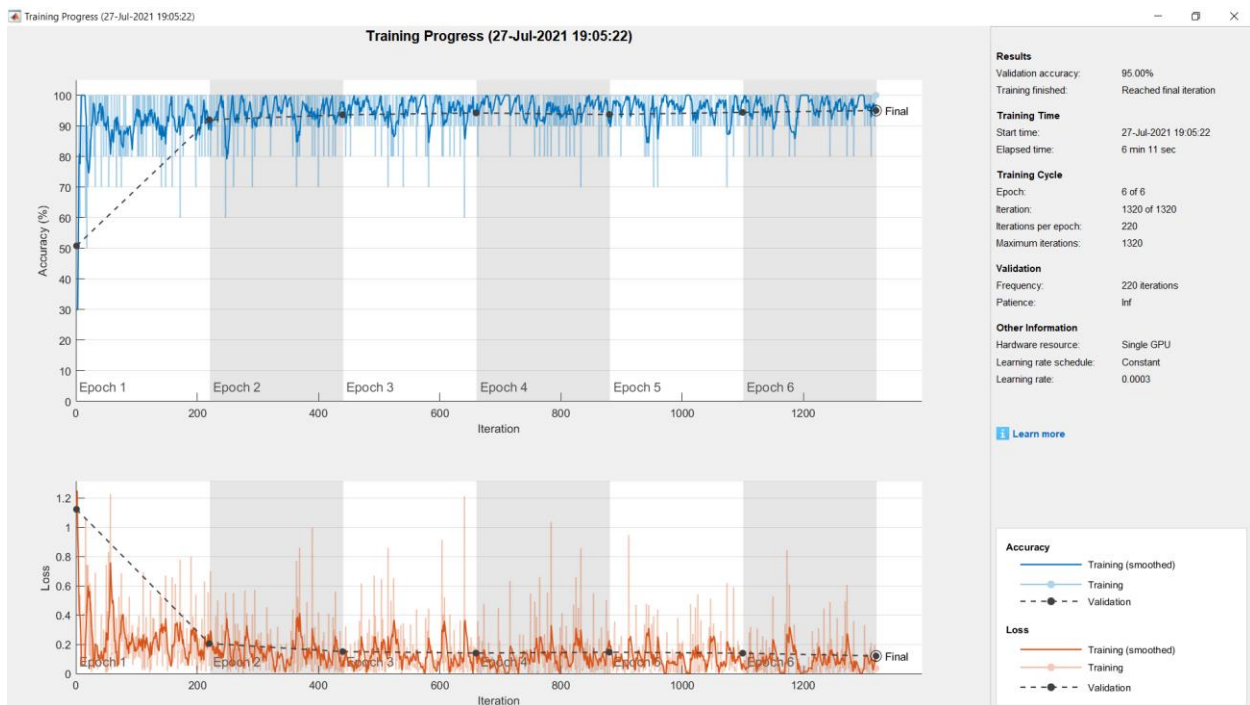
Figure 29: Respective transfer learning progress graph of accuracy and loss from Section 2.3.1. Number of iterations/Number of epochs: 1320/6, Batch size: 10, Learning rate: 0.0003, Training time (Single GPU): 6 minutes 11 seconds.
