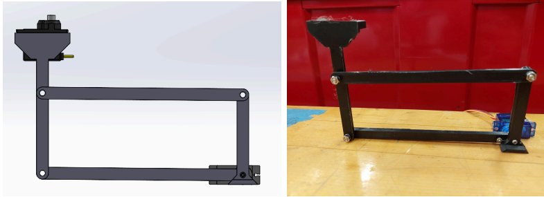
Figure 6.12: CAD (left) and prototyped (right) versions of the four-bar lift
