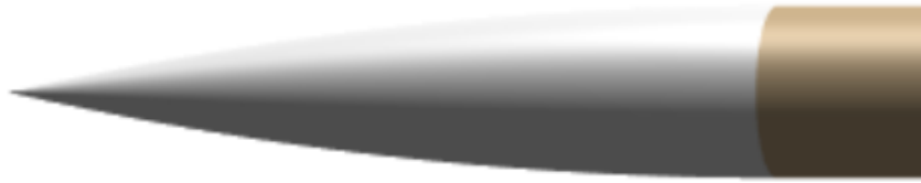
Figure 14: Example of long ogive nose cone
