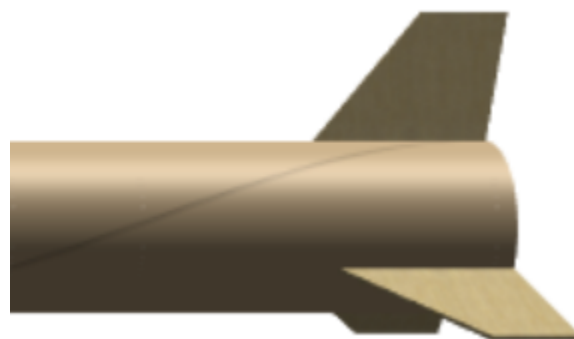
Figure 13: Example of swept fins
