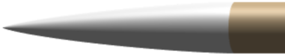
Figure 17: OpenRocket example of Von Karman nose cone
