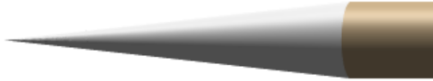
Figure 16: OpenRocket example of conical nose cone
