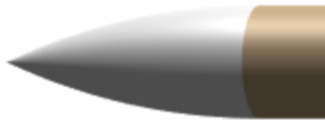
Figure 15: OpenRocket example of short ogive nose cone
