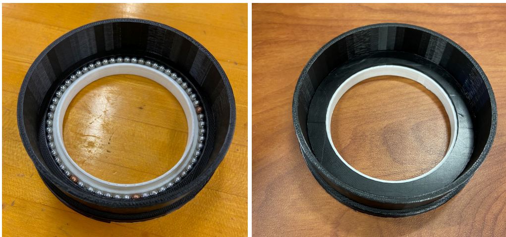
Figure 6.6: Prototype of 3D printed custom bearing
